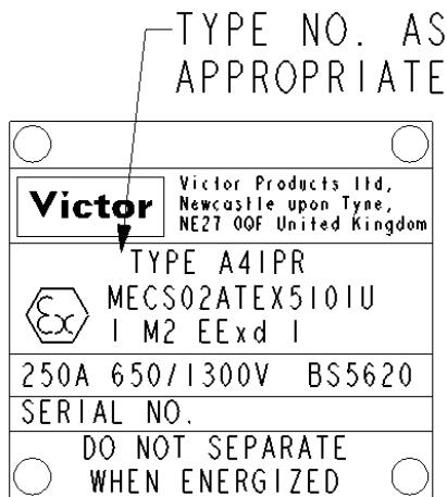
NAMEPLATE DETAIL RESTRAINED PLUGS
