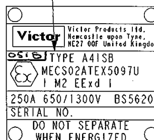
NAMEPLATE DETAIL BOLTED SOCKETS
