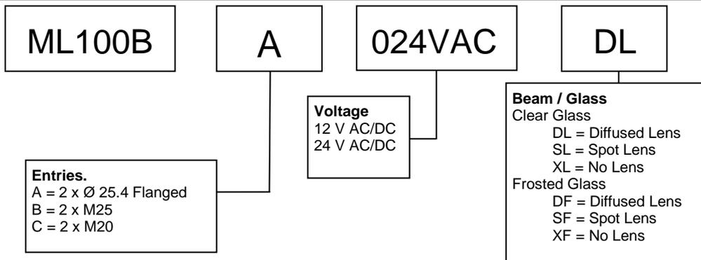
**EXAMPLE:** ML100BA012VDCDL = ML100 LED Machine Light in Brass suitable to take 2 off 25.4 mm diameter flanged glands. Voltage is 12V AC/DC with Diffused lens fitted, clear glass.
