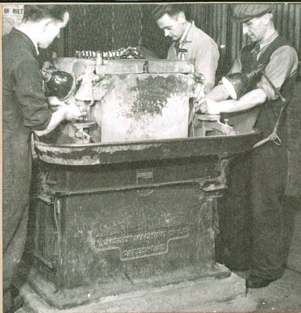
A four wheel grinder for dressing drill bits to profile after welding.
